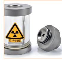
The innovative design of the lid and its fixing system with 2 O-rings guarantees secure sealing of the vial shields. A removable cap, also fitted with an O-ring, allows the preparation to be completely isolated when not in use and prevents leakage.
